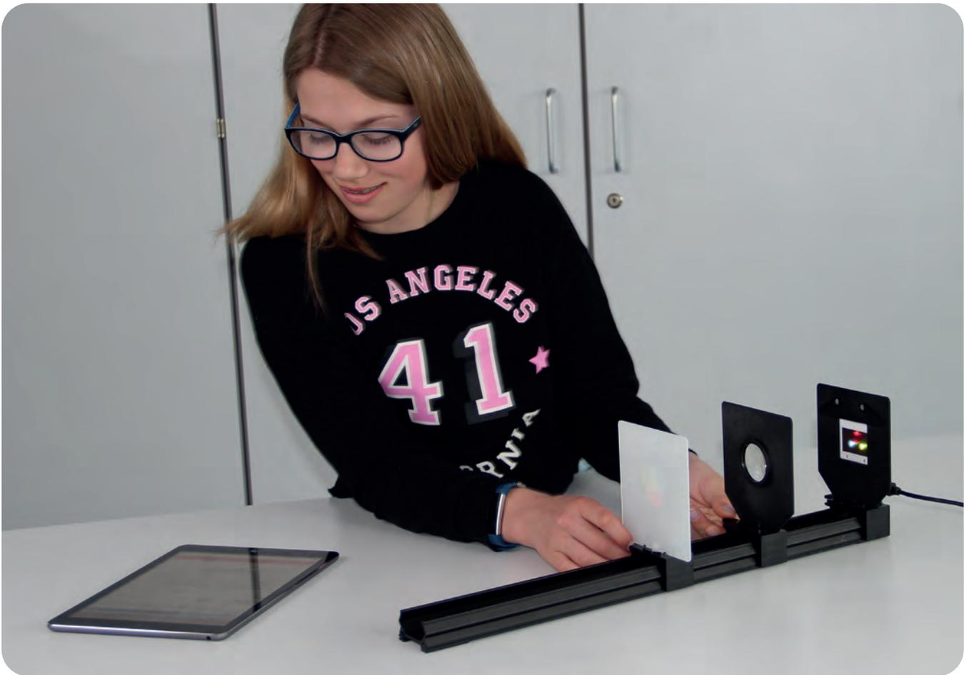
LP5.2.3.4 Additive mixing of three light colours
